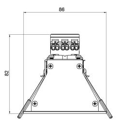
Dimensions: 1000 x 82 x 86 mm Total power: 30 w Luminaire luminous flux: 3000 lm Luminaire efficacy: 100 lm/w Weight:1.6Kg
